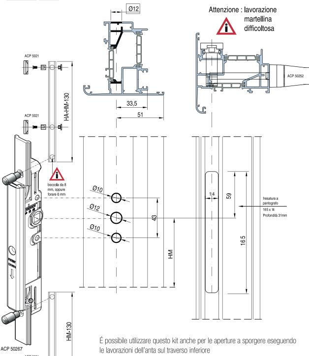
It's possible to use this kit even in top-hung open out windows, making the machining sill
