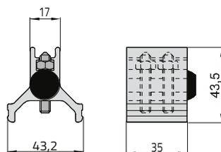
Back stop in aluminium with rubber buffer.
